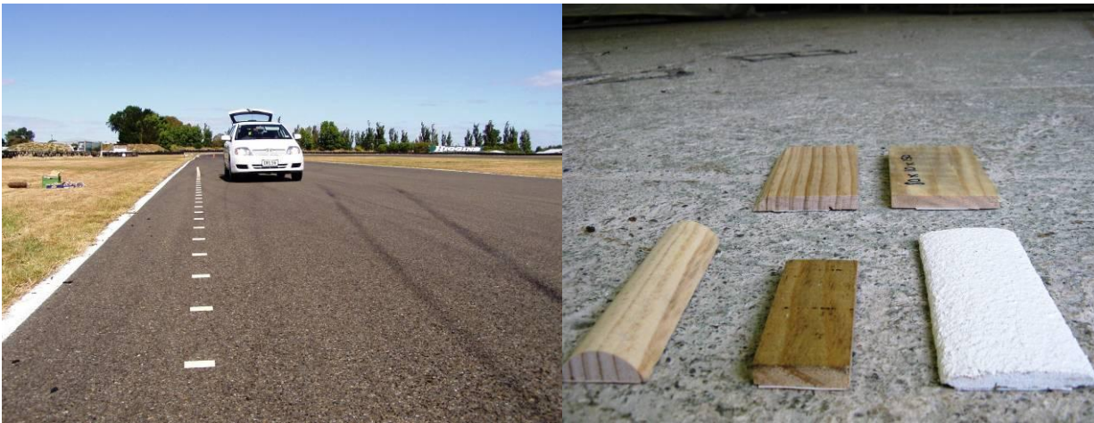
Figure 5 The test car next to a line of test blocks on the Manfeild race track and a selection of four wooden test blocks and a thermoplastic test block that were used in the testing. The car is shown facing the opposite direction to that travelled during the testing.
