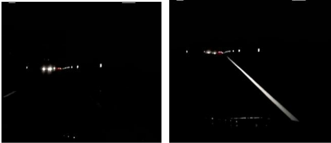
Figure 5 Standard road marking (left) vs All Weather marking (right) during rainfall
